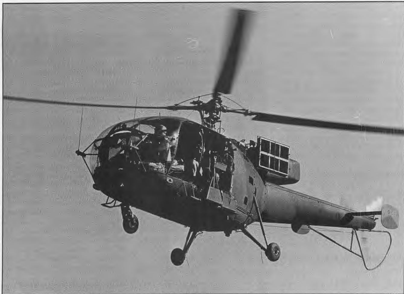
Logistically strapped by international embargo, Rhodesia pressed into service every available aircraft for insertion, including these aging Alouette IIIs. By running shy on fuel on the haul back, they could carry 500 pounds of captured weapons and a few men. Photo: SOF file
